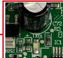
LED1: Drive failure indicator
