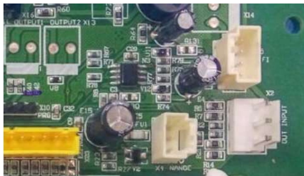
Figure 3 main control board
